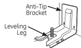
To reduce the risk of tipping the range, the range must be secured by a properly installed anti-tip bracket. See installation instructions shipped with the bracket for complete details before attempting to install.
